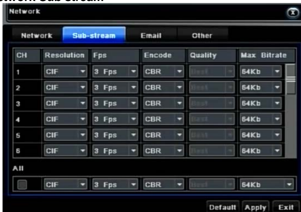
Pic 2.4.6.2 Network Sub stream
